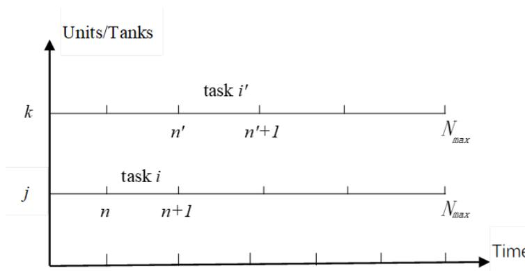
**Figure 3.** Continuous-time representation for whole refinery processes
