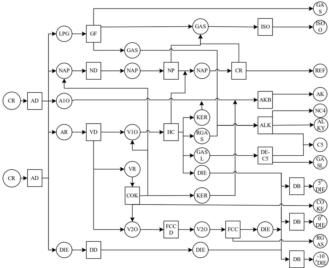
**Figure 1.** Superstructure flowchart for whole refinery processes
